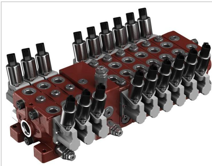
Additionally, on mini-excavators, where up to 3 or 4 simultaneous operations are common, it is very easy to run into the problem of flow saturation. It happens every time that the operator is demanding more oil flow than the pump can deliver: the Flow Sharing helps to guarantee movement contemporaneity, but it results in a
